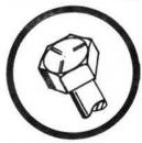
A GRADE 5 HEAT TREATED BOLT CAN BE IDENTIFIED BY THREE LINES INDICATED ON THE BOLT HEAD AS SHOWN AT LEFT.
